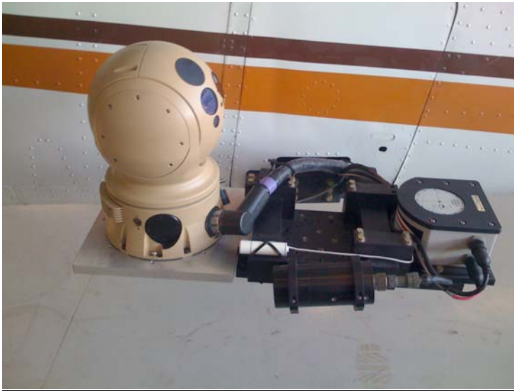
FLIR TALON mounted on AeroComputers test aircraft
